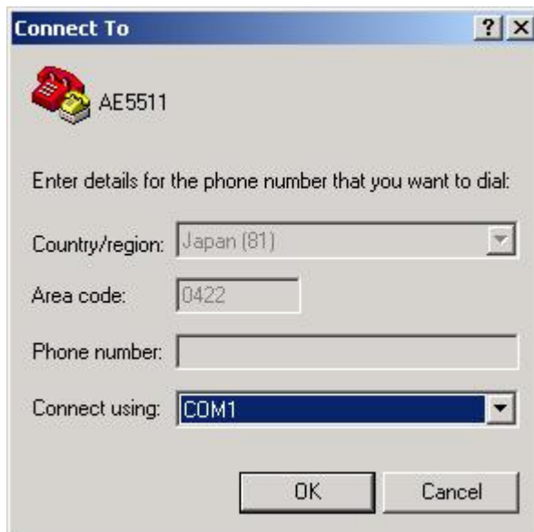
Figure 4.10-4 Connection setting screen
